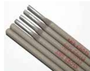
ISONIC: ELECTRODO AWS A5,1 PREMIUM E6013 5/32" 4,0MM X 350MM (CHE40) (FÁBRICA ATLANTIC)
