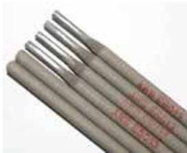
ISONIC: ELECTRODO AWS A5,1 PREMIUM E6010 1/8" 3,2MM X 350MM (CHE425G) COLOR ROSA
